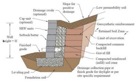
visual enhancement at the face of the wall. For reinforced SRW systems, the interface between SRW units also provides a connection point for the soil reinforcement.
