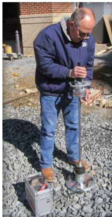
Figure 22. Testing base stiffness using light-weight deflectometer.
