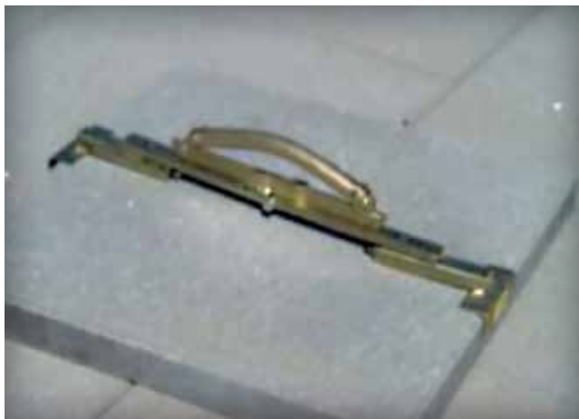
Figure 9. Single hand scissor clamp for lifting small and thin paving slabs
