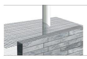
**IMPORTANT** When a fence is within the Reinforce Soil Zone, install Sonotubes during wall construction. This will prevent damage to the grid resulting from sleeves being punched or augured through the reinforced zone. Wrap the geogrid around the Sonotube. Cut only the cross members of the grid, not the strength members. Provide at least 25mm (1") clearance between the inside of the sleeve and the outside of the post to allow for mortar and grout.
