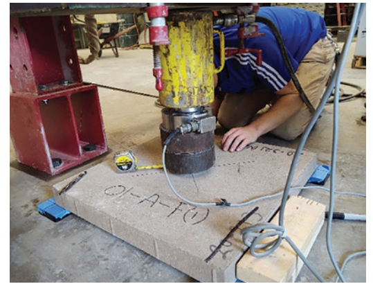
Full-Size Slab, Corner Support Testing
