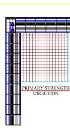
FIRST COURSE ENSUREING IT IS PLACED WITHIN  $25\mathrm{mm}$  [1.0"] OF THE FACE OF THE BLOCK AND RUNNING ALONG ON EACH WALL COURSE THAT GEOSYNTHETIC REINFORCEMENT IS SPECIFIED, LAY THE GEOGRID UP TO CORNER OF THE WALL, THE BACK OF THE ADJOINING WALL PRIMARY STRENGTH
