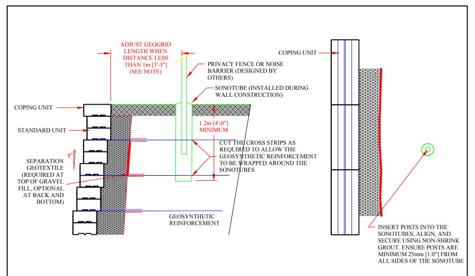
NOTE: WHEN THE PRIVACY FENCE OR NOISE BARRIER IS AT LEAST 1m [3'-3"] BACK FROM THE WALL FACE, GENERALLY NO ADDITIONAL REINFORCEMENT IS REQUIRED. WHEN THE PRIVACY FENCE OR NOISE BARRIER IS INSTALLED WITHIN 1m [3'-3"] OF THE WALL FACE, THERE MAY BE SOME LOAD TRANSFERRED TO THE WALL FROM WIND, SNOW, OR PEDESTRIANS; ADDITIONAL REINFORCEMENT AROUND THE SONOTUBES AND/OR DEEPER SONOTUBES MAY BE REQUIRED.
