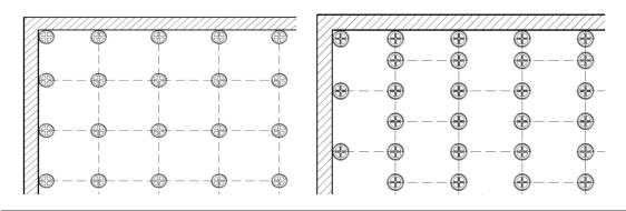
NOTE TO READER – the above equation is based on the slab being <u>fully</u> suspended on both ends by metal rods similar to a one-way slab in building construction. In reality pedestal set products are suspended at the four corners, similar to a flat slab, but there are no simple calculations to model this scenario. As of the last update of this document, ICPI, to which Oaks is a member, is working on developing ways to properly model and evaluate pedestal set materials.
