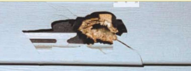
Above photo shows exit point of vinyl sided wall after bullet has passed through corner (i.e. two complete walls).
