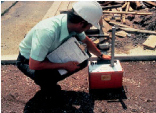
Figure 6. Monitoring of base compaction during construction minimized the likelihood of settlement later.
