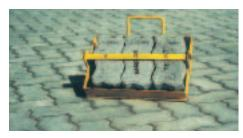
Figure 12. A sample panel of good, marginal, and unacceptable pavers used by factory and site personnel provided visual acceptance criteria of the paver surface texture. This was part of a comprehensive program of quality control and quality assurance measures implemented throughout the project.
