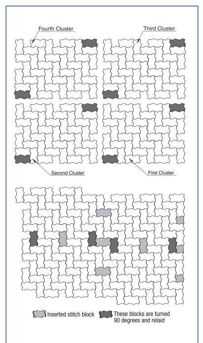
Figure 11. Upon machine placement of each cluster on the bedding sand, pavers at the corners were re-oriented and stitching pavers inserted or turned to create a consistent, fully interlocking surface across the pavement.
