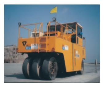
Figure 18. This 44-ton (40 T) machine rolled the completed surface of the pavers (prior to application of the sealer) to prove that they were seated and that the joints were full of sand.
