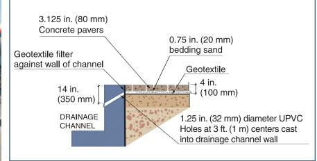
the pavement, the drain holes dissipate excess water in the bedding sand, thereby reducing the chance of pore pressure build-up and sand loss through the joints. To ensure that the bedding sand was not washed away through the weep holes, the geotextile continued up the face of the drainage channels to  $^{3}/_{8}$  in. (10 mm) below the surface.
