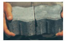
Figure 14.The left half shows a saw-cut paver with a chamfer on the cut edge.The right half shows a paver with rough edges cut with a manual splitter. No pavers at Hong Kong were cut with a splitter. Saw-cut pavers and chamfers eliminate risk of ingestion of chipped concrete into jet engines.
