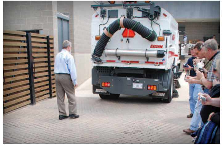
Maintenance workshop at Morton Arboretum demonstrates equipment that effectively cleans PICP openings
