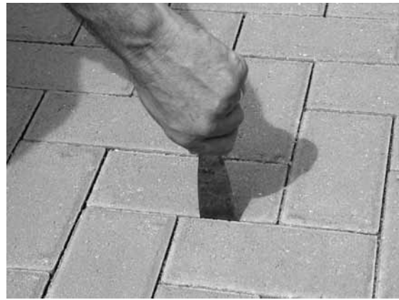
Figure 13. A simple test with a putty knife checks consolidation of the joint sand.
