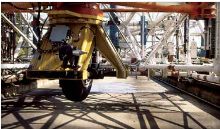
Figure 7. Test equipment for evaluation of the friction properties of concrete pavers at NASA's Aircraft Dynamics Landing Facility (ADLF) in Langley, Virginia
