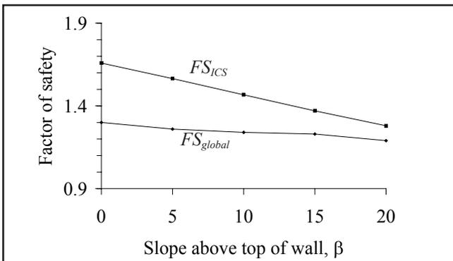
**Figure 5**—Effect of Slope Above Top of Wall
