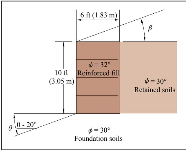
**Figure 3**—Typical Section for Figures 4 and 5
