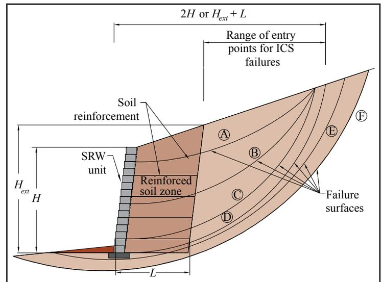
**Figure 1—Global Stability Failures**
